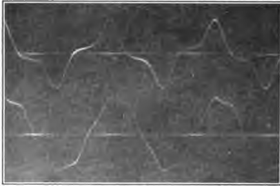
FIGS. 100 and 101. Exciting current of delta-connected transformers. Upper curve, transformer current. Lower curve, line current.
